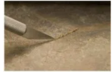
Sedimentary rock (slate) can be clay, shale or quartz based varying in hardness from 3 to 7. This image shows a slate equivalent to a softer marble.
