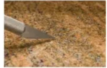
Hardened steel and quartz (granite) have the same hardness rating.
