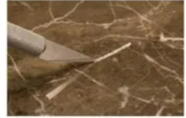
Calcite (marble) is rated at a 3 for hardness.
